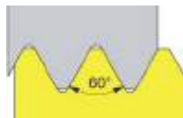
Rosca Externa Perfil Parcial Partial Profile External Thread Filetage Extérieur Profile Partiel
