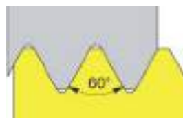
Rosca Externa Perfil Total Full Profile External Thread Filetage Extérieur Profile Totale
